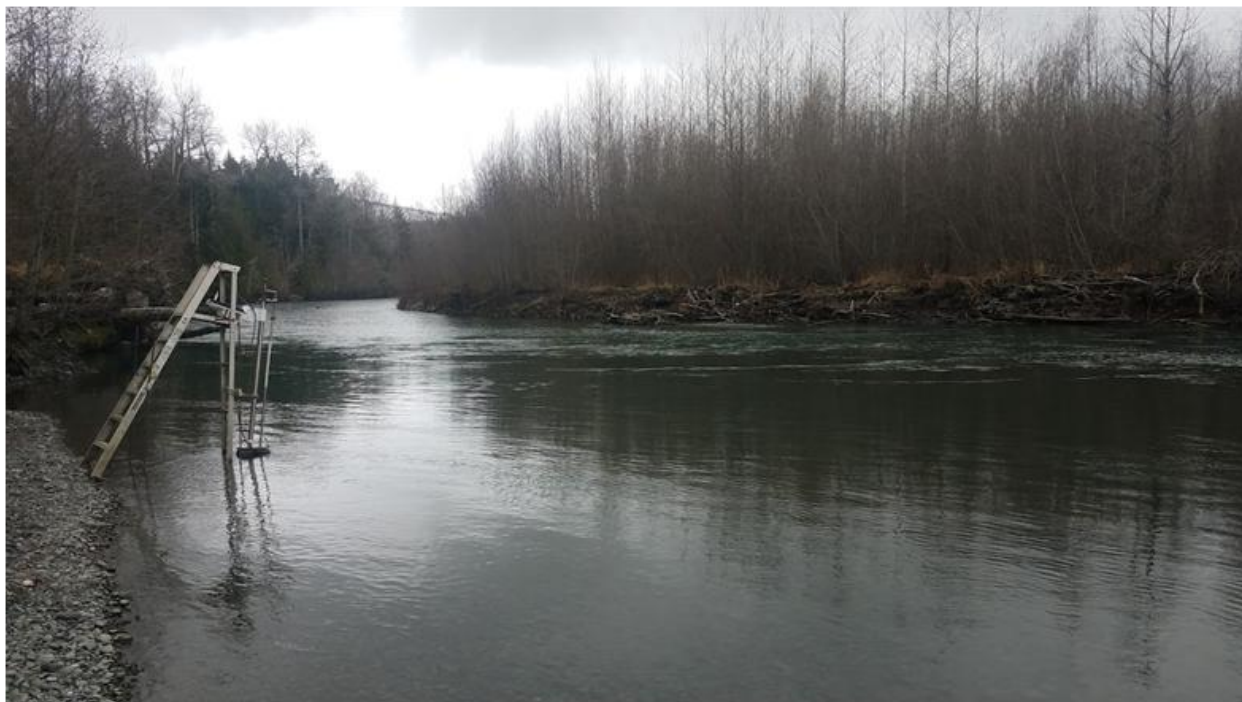
Figure 3. East Channel or Mainstem SONAR site looking upstream. The SONAR is attached to the pole mount which is in turn attached to the ladder.
